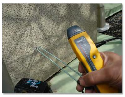
Moisture readings were taken in a number of locations indicated by the site map below. Locations were chosen if they were considered at risk due to either conditional appearance or the potential vulnerability of a specific construction method or component. Another reason was to confirm that past remediation was performing as desired and we re-checked some locations that had been tested in the past. All of the
