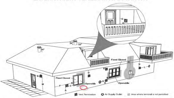
Minimum clearance is 12" (30cm) from a window or door that may be opened. The window in question is approximately 36" (90cm). Grey areas above are the "no installation" zones. (Information provided by Regency P36D-1FireplaceInstallation Manual for Zero Clearance Direct Vent Gas Fireplaces in stated accordance with CSA B149.1, *Natural Gas and Propane Installation Code and ANSI Z223.1/NFPA 54, National Fuel Gas Code, Page 21.*)
